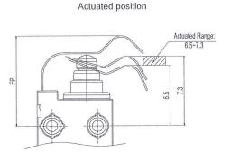
B3. The switch will be broken, if you give larger stress than specified (chapter 5.6/5.7). Take most care not to let the switch given with larger stress than specified.
